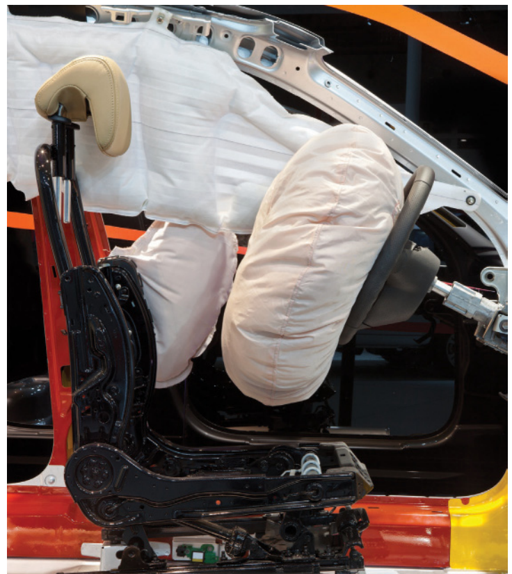
Figure 1-7 Side airbags and air curtains pose a hazard to responders, if the devices did not activate in the collision. Note: See the Access: First on Scene—Rapid Vehicle Entry Provider Manual from ITLS for more information about rendering nondeployed airbags safe. (testing, Shutterstock)
